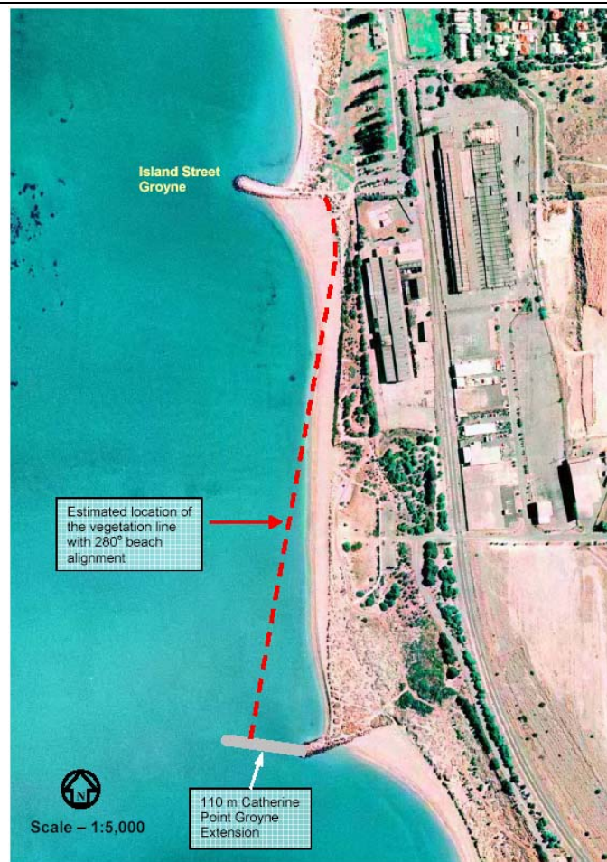
Figure 3: Initial estimated shoreline position if the Catherine Point Groyne is extended by 110 metres (MRA, 2006). Note, it has been recently estimated that a shorter groyne extension of 30m is appropriate to extend the beach (MRA, 2007).
