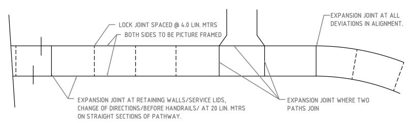
LOCK JOINT MUST ONLY BE INSTALLED ON CLEAN SAND FILL. EVENLY SCREEDED. WATERED AND WELL COMPACTED TO A MINIMUM DEPTH OF 500mm AND 95% MODIFIED MAXIMUM DRY DENSITY. (OR TO ENGINEERS SPECIFICATIONS) CONCRETE SHOULD BE AT LEAST 32mpa.
