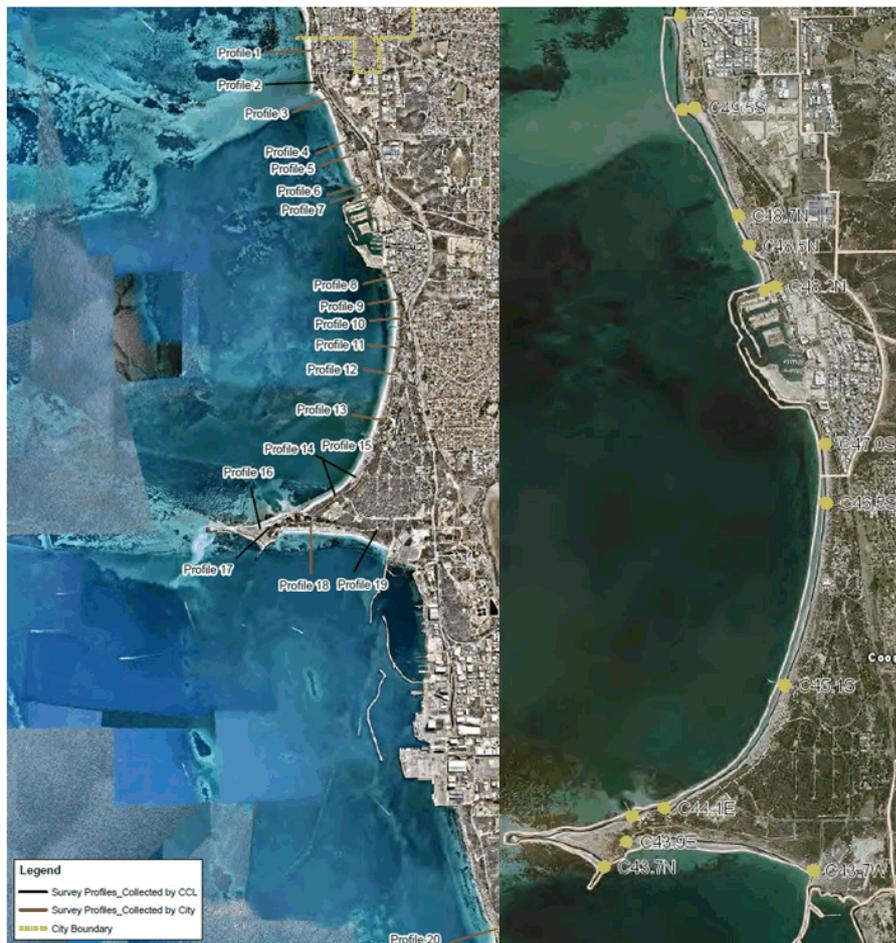
**Figure 11 Coastal monitoring program beach profile locations (Left) and photo monitoring locations (Right)**
