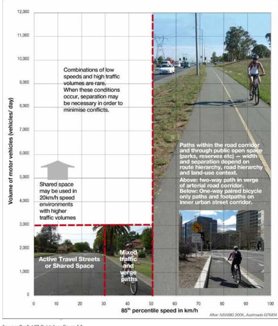
Figure 7.2: Separation of cyclists and motor vehicles by speed and volume
