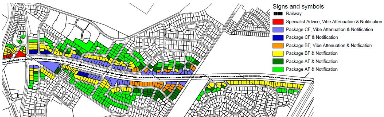
Figure 7: Freight Train Noise & Vibration Impacts (Ground Level) Source: Figure 7.1 from the Freight Train Noise & Vibration Assessment Bibra Lake & South Lake
