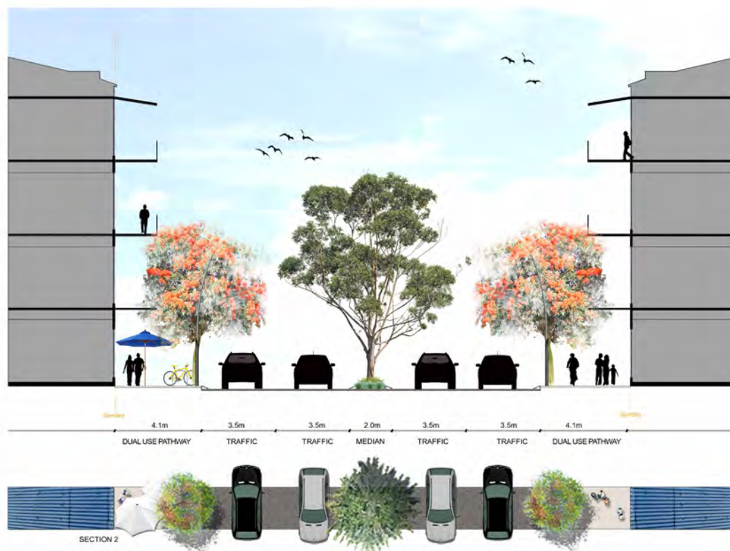
Figure 41_Possible Cross Section through Cockburn Road
