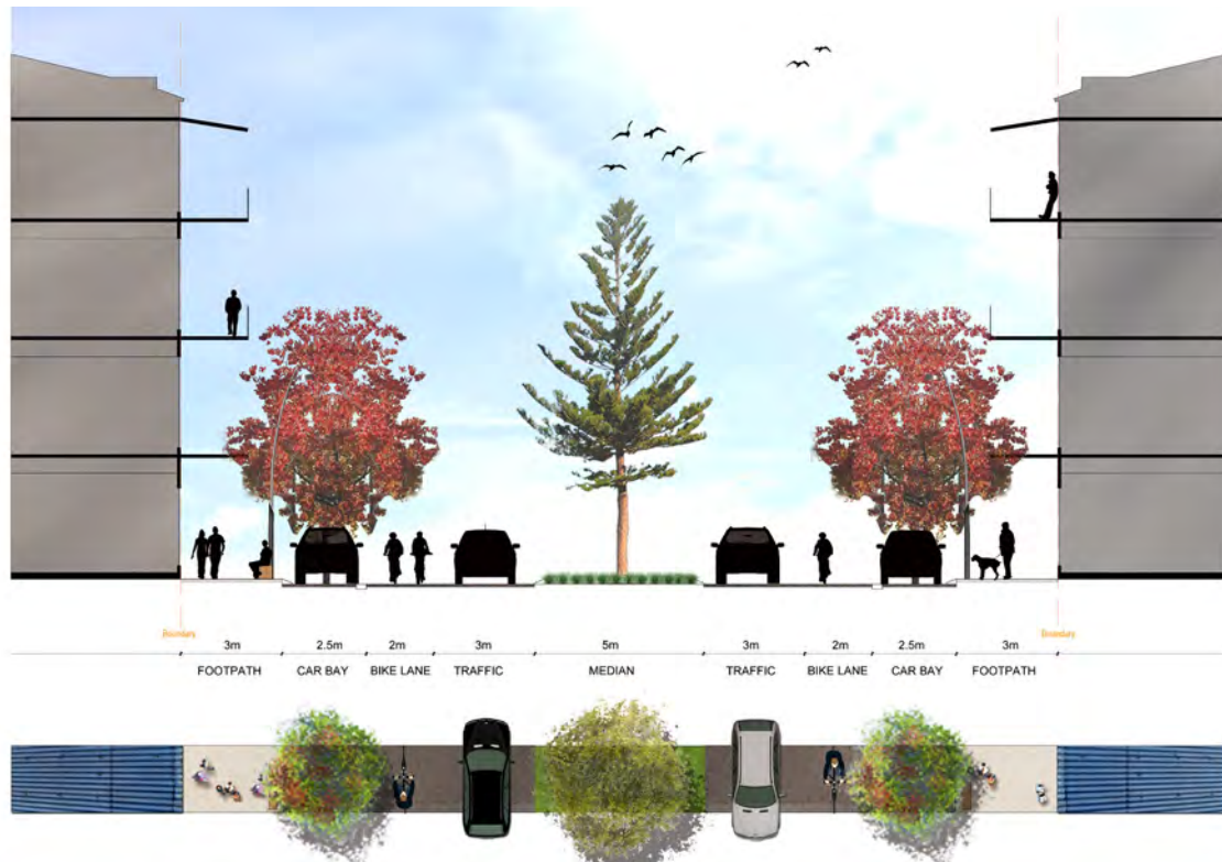
Figure 36_Possible Cross Section through Main Street with median
