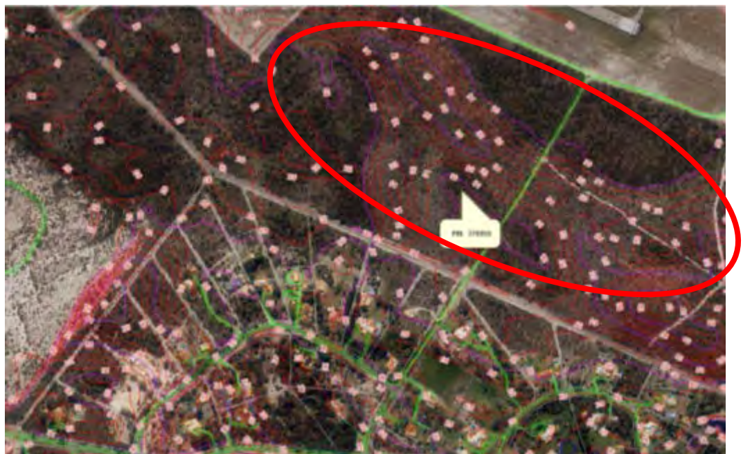
Map showing how Precinct 6 will be earth worked to likely remove ridge, creating same level (28-30 contour) as properties adjoining
