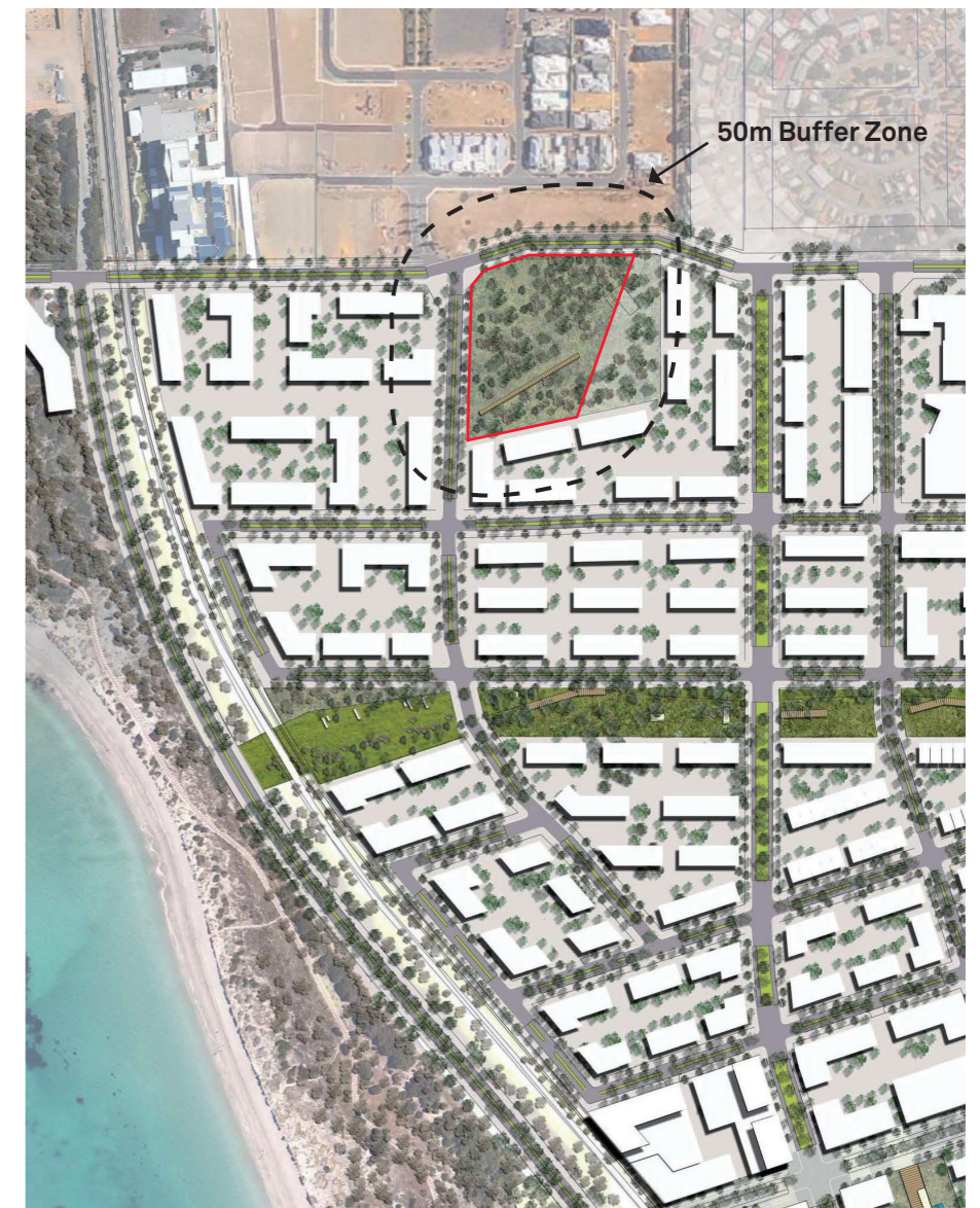
Figure 79_Waste water pump station buffer no sensitive land uses permitted within this area unless approved as part of the local structure plan
