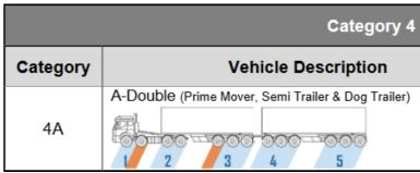
Figure 23 RAV4 network approved vehicle configuration (source: Main Roads WA)
