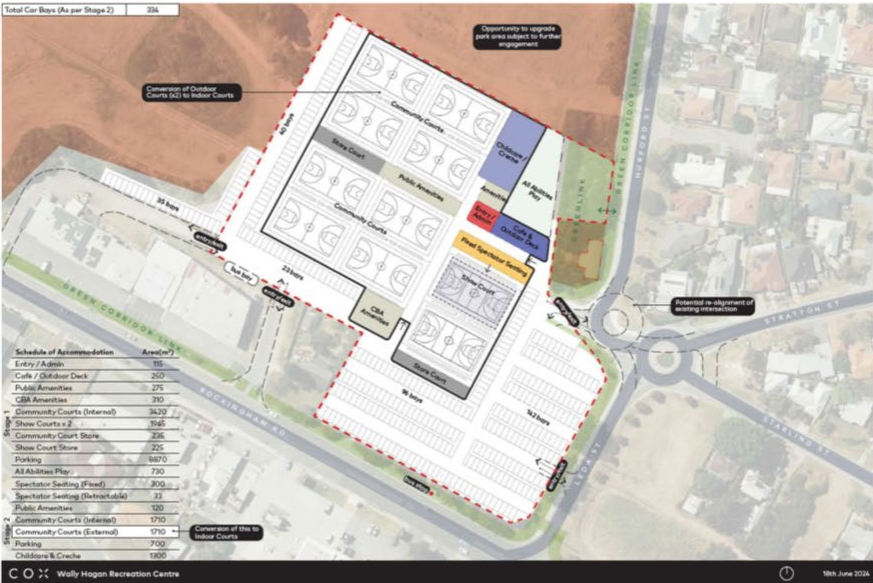
Image 16: WHRC Concept Plan – Stage 3. Stage 3 of the project, should it occur, is the conversion of the two outdoor courts into indoor courts.
