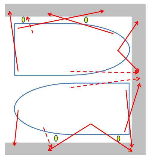
Additional breast and spring lines are highly recommended for 12m+ vessels.
