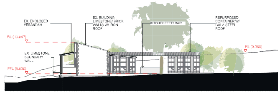
Post Office South Elevation 1:200
