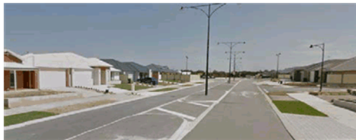
Figure 8. Residential streetscape (Hammond Park) where hardscaping dominates due to insufficient space for street trees and numerous breaks in the median for access to crossovers
