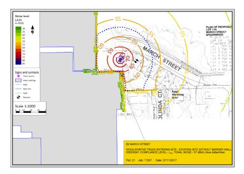
It has been suggested by an acoustic consultant that the construction of a 4m acoustic barrier wall on the east side of the existing loading dock ramp is expected to block the visibility of trucks accessing the loading dock. Further, the construction of a barrier wall perpendicular to the front boundary 6m in length, 3m in height and setback 4m from the front kerb may also be required. The construction cost of the noise wall is estimated to be in excess of \$100,000.
