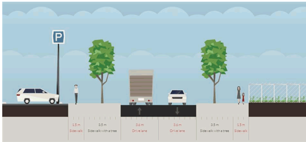
Figure 5.1: North Lake Rd to Lot 55 Crossover Cross-section
