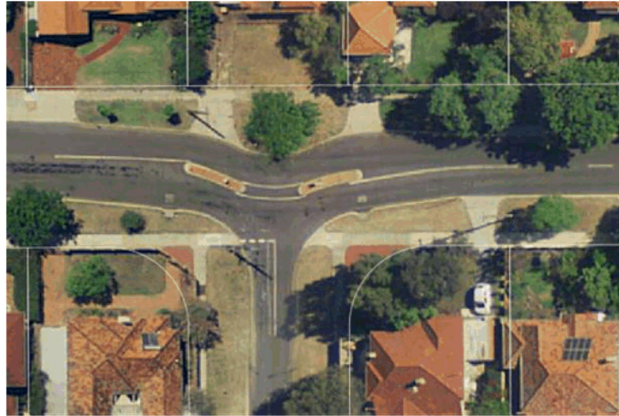
Figure 4 – Typical T-Junction Slow Point Installation
