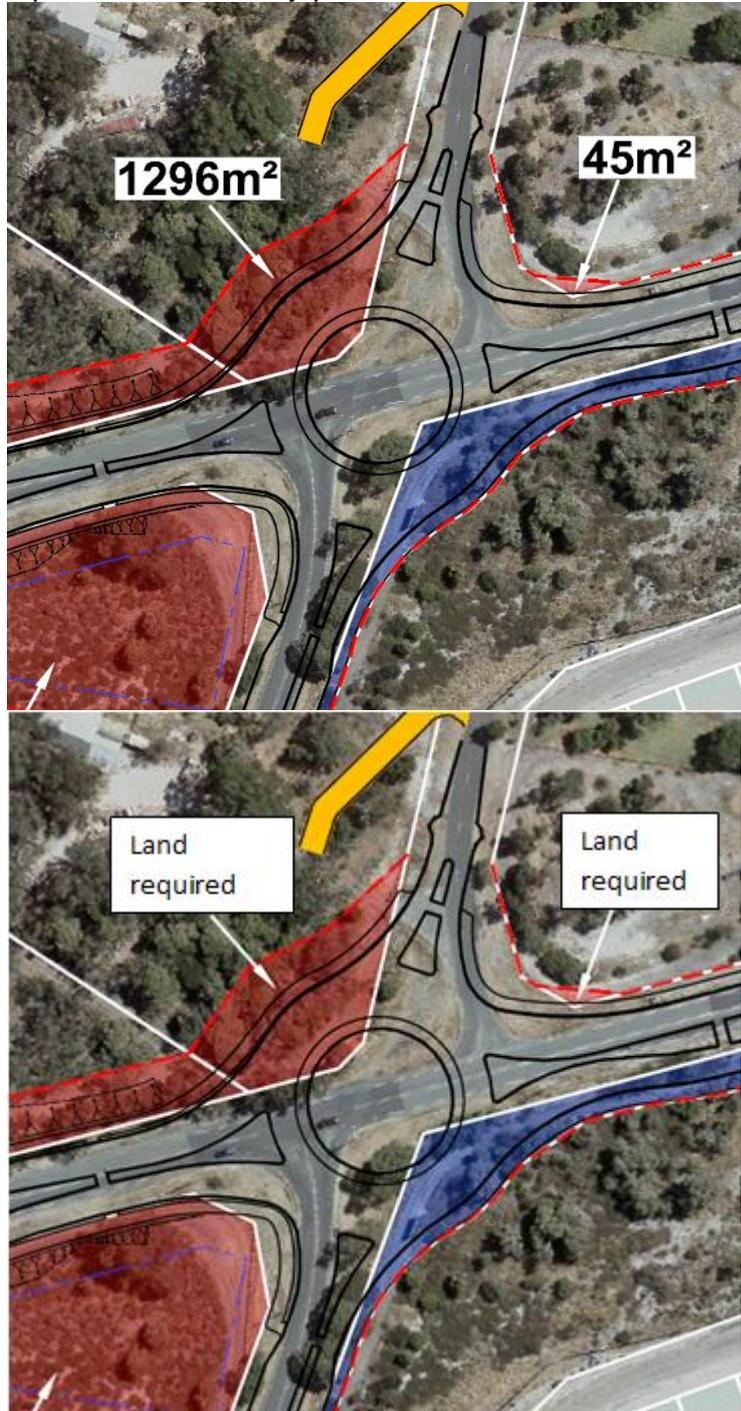
Option 2 - an offset positioned roundabout
