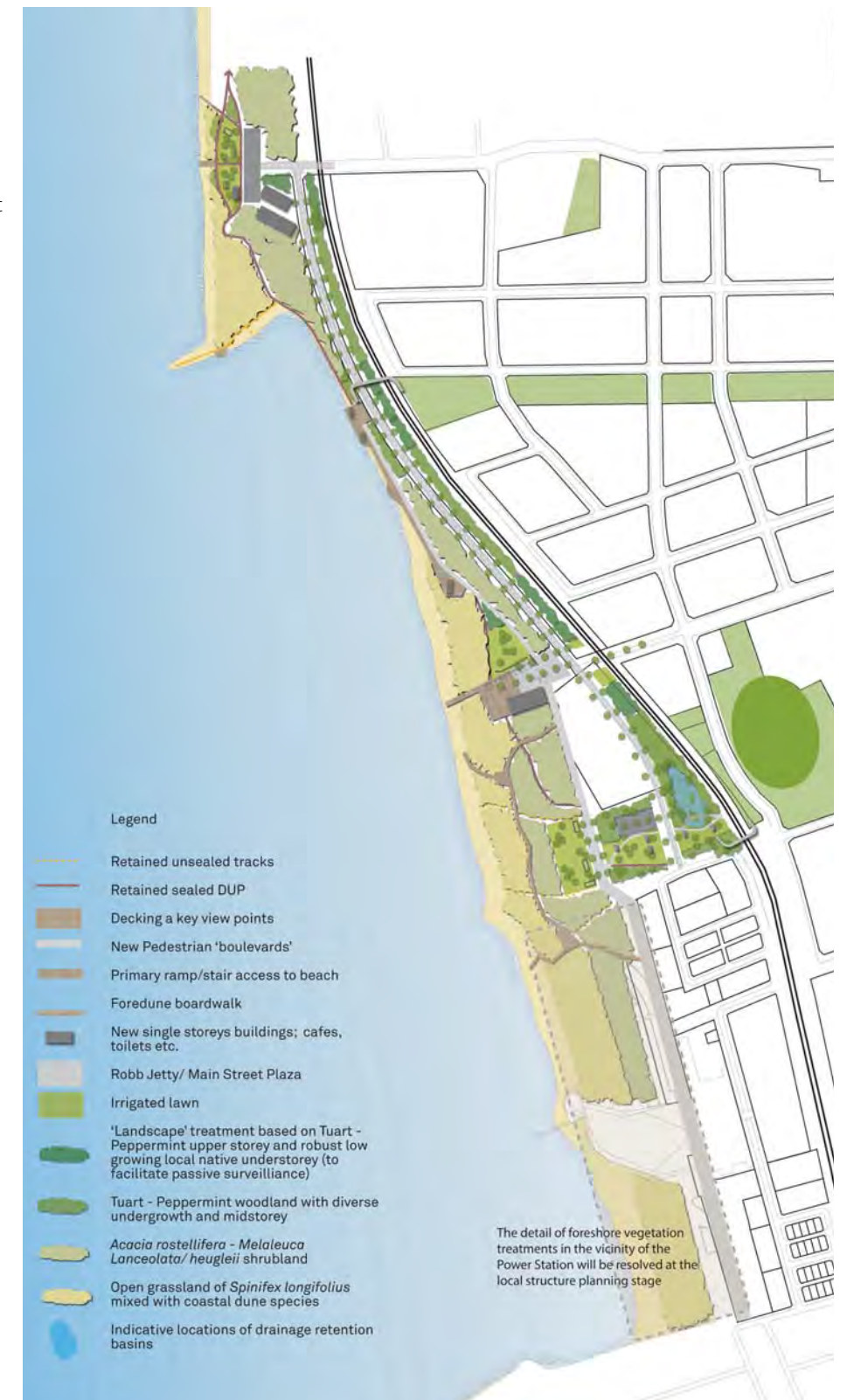
Concept Image indicating Infrastructure and vegetation treatments for the Seawall Coastal Protection Option
