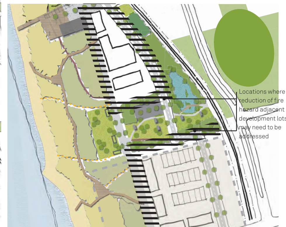
Figure 5.19 Locations where reduction of fire hazard adjacent development lots may need to be addressed
