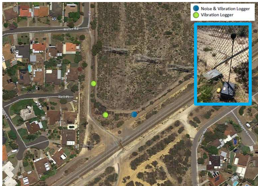
Figure 8: Location of the Noise and Vibration Data Loggers on Subject Site Source: CoC Lakes Revitalisation Strategy Background Report (December 2015) – Acoustic Assessment (July 2016)
