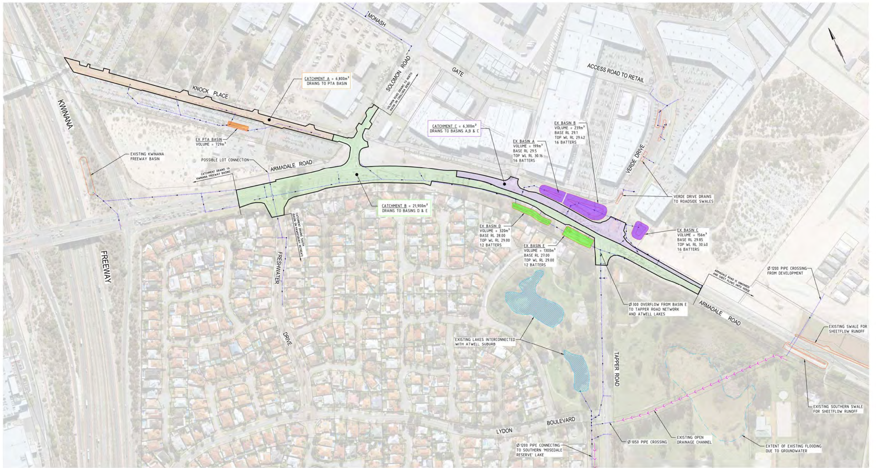
E15084-043-SK-C-0010 (Rev A) Existing Drainage Catchments and Drainage Network North Lake Road Realignment - Kwinana Freeway to Fraser Road Scale 1:2000 at A1
