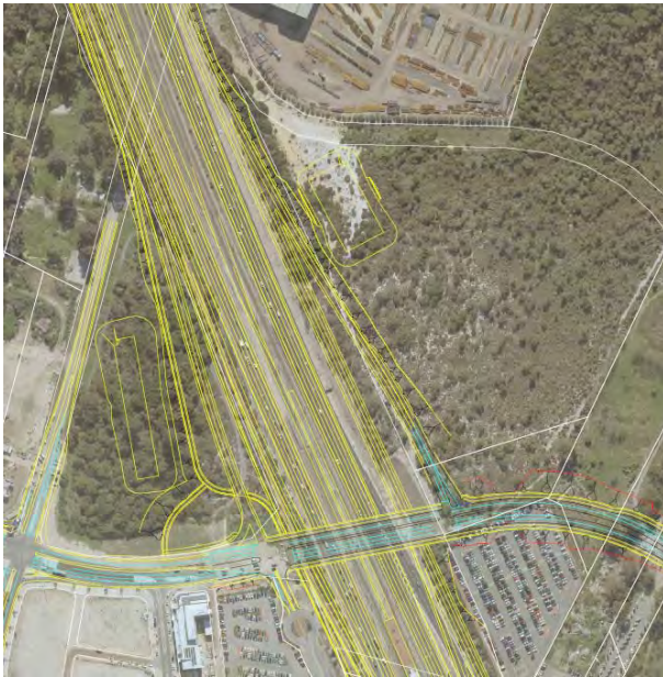
Plate 3 and 4: Concept Drainage Plans for Lot 9500 (left, MRWA 2016) and the CCE Structure Plan Area (right, BG&E 2017)
