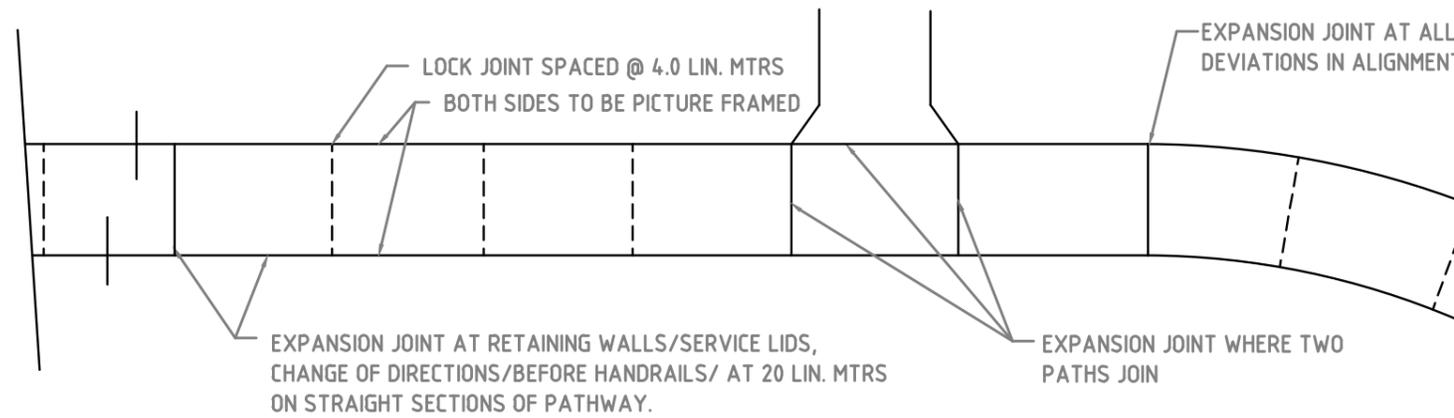
LOCK JOINT MUST ONLY BE INSTALLED ON CLEAN SAND FILL, EVENLY SCREEDED, WATERED AND WELL COMPACTED TO A MINIMUM DEPTH OF 500mm AND 95% MODIFIED MAXIMUM DRY DENSITY. (OR TO ENGINEERS SPECIFICATIONS) CONCRETE SHOULD BE AT LEAST 32mpa.
