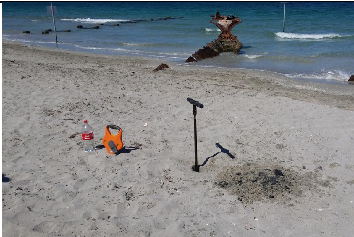
Photo 2. Sub-surface probing by hand auger, observed black sand at the bottom at about 0.8 m
