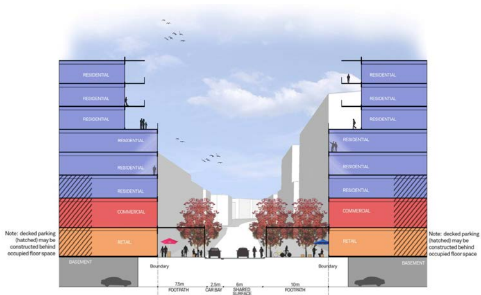
Figure 05_Typical cross section for activity centre development
