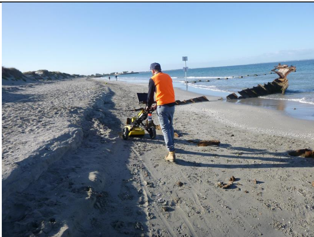
Photo 8. GPR Scanning just outside of the middle beam, looking toward south
