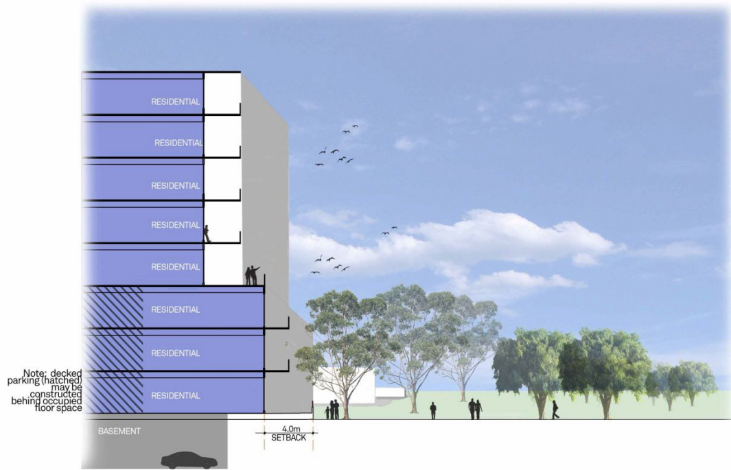
Figure 10_Typical cross section of high density residential directly adjoining public open space
