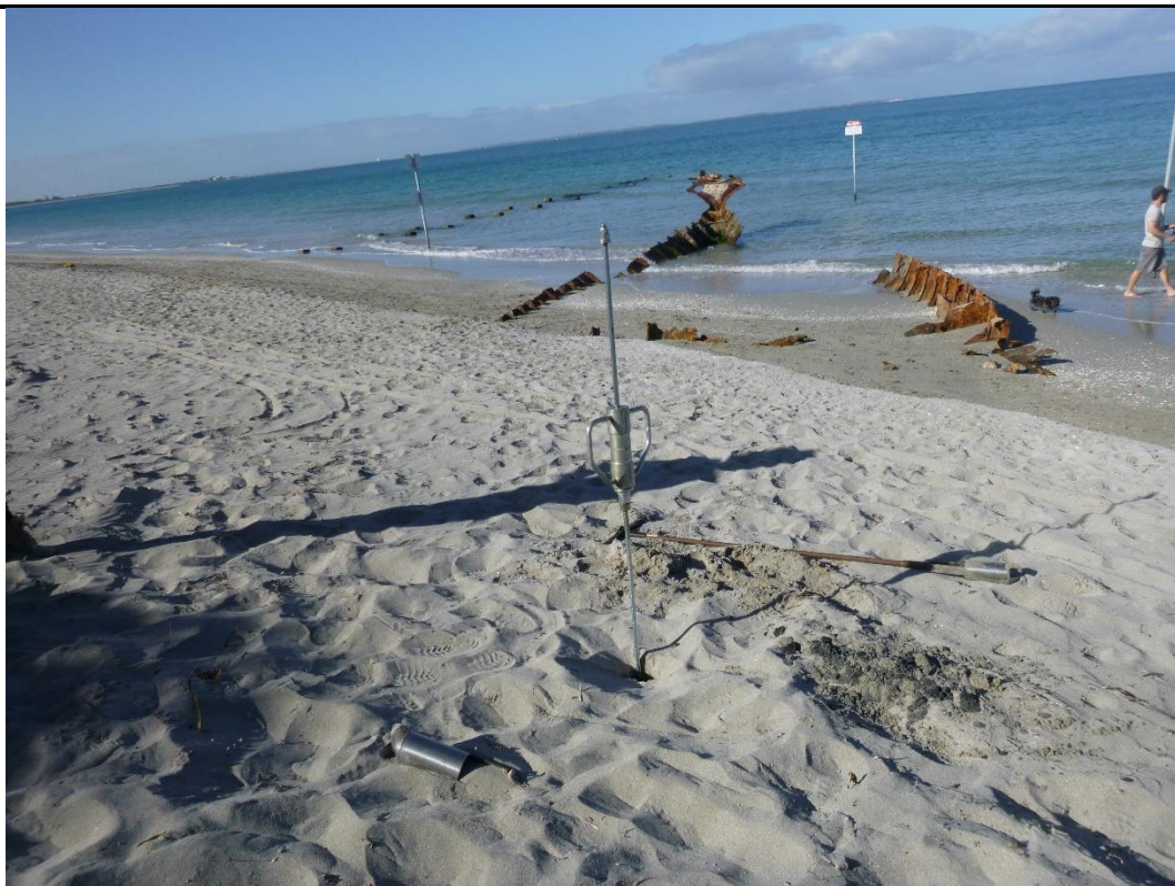
Photo 4. Sub-surface probing and DCP test observed black sand at the bottom at about 1.8 m
