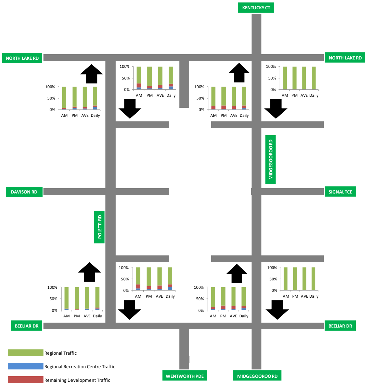
Figure 28 Volume contributions on Poletti Rd and Midgegooroo Rd
