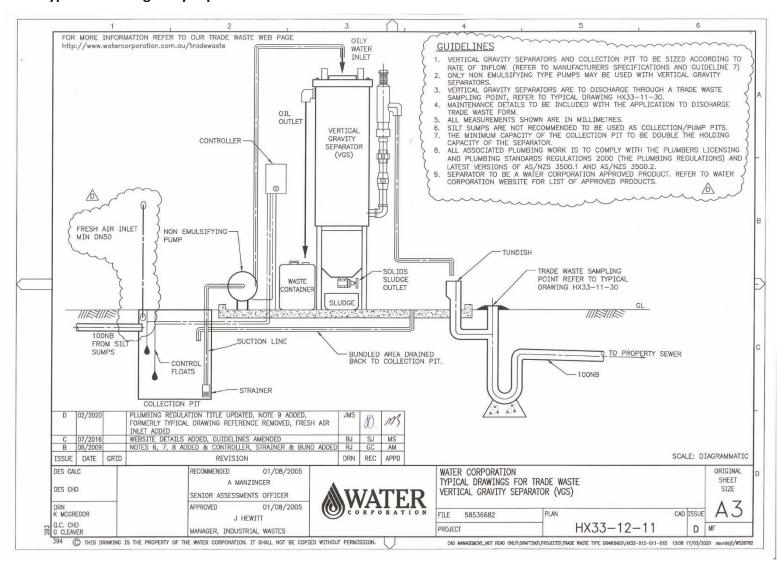
**Diagram HX33-12-11,** Typical vertical gravity separator. Source: www.watercorporation.com.au Image is not to scale.
