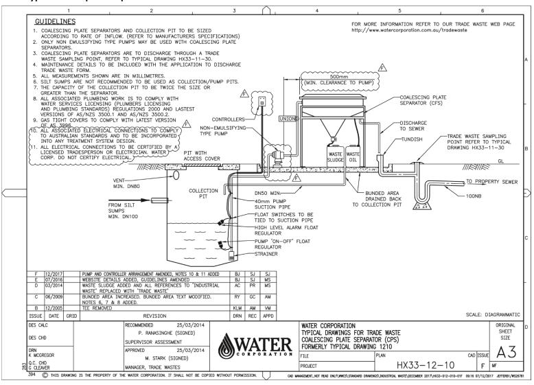
**Diagram HX33-12-10,** Typical small plate separator. Source: www.watercorporation.com.au Image is not to scale.
