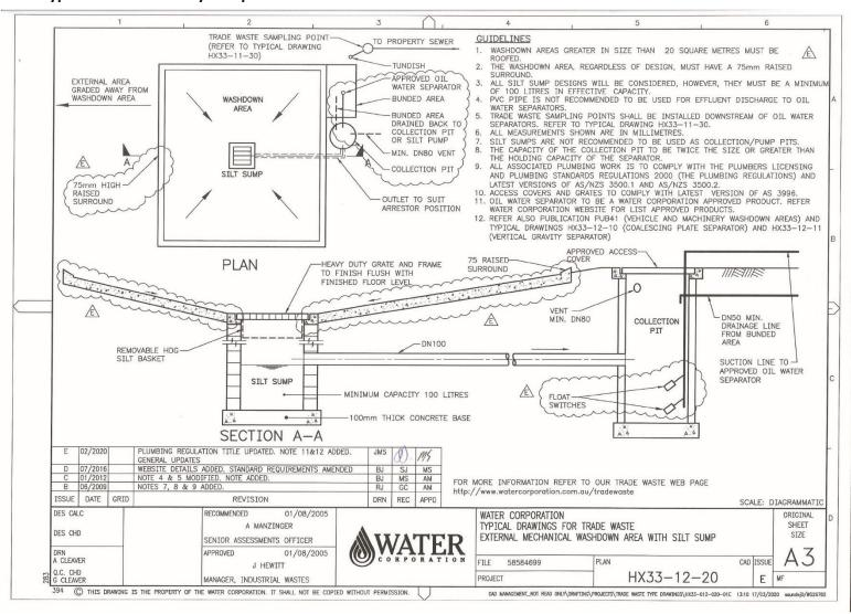
**Diagram HX33-12-20,** Typical washdown bay setup. Source: www.watercorporation.com.au Image is not to scale.
