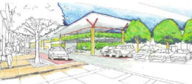
AFTER – More shade, wider footpaths, narrower roads with raised pedestrian crossings. Parallel parking to protect footpath dining facilities and slow traffic without the need for frequent and severe speed humps. Night market allows a greater variety of businesses to open up and creates a venue for social gathering. Access to drive-through businesses restricted to Rockingham Road only, creating a calmer environment dominated by pedestrians.
