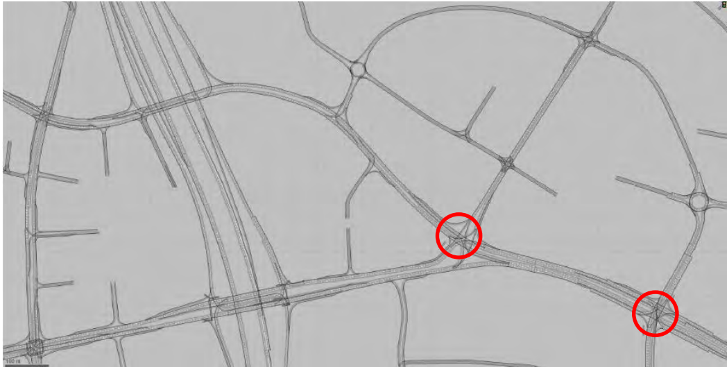
Figure 4: Modified City of Cockburn Developed Option (Shown in red - intersections proposed to be grade separated). Current preferred route.
