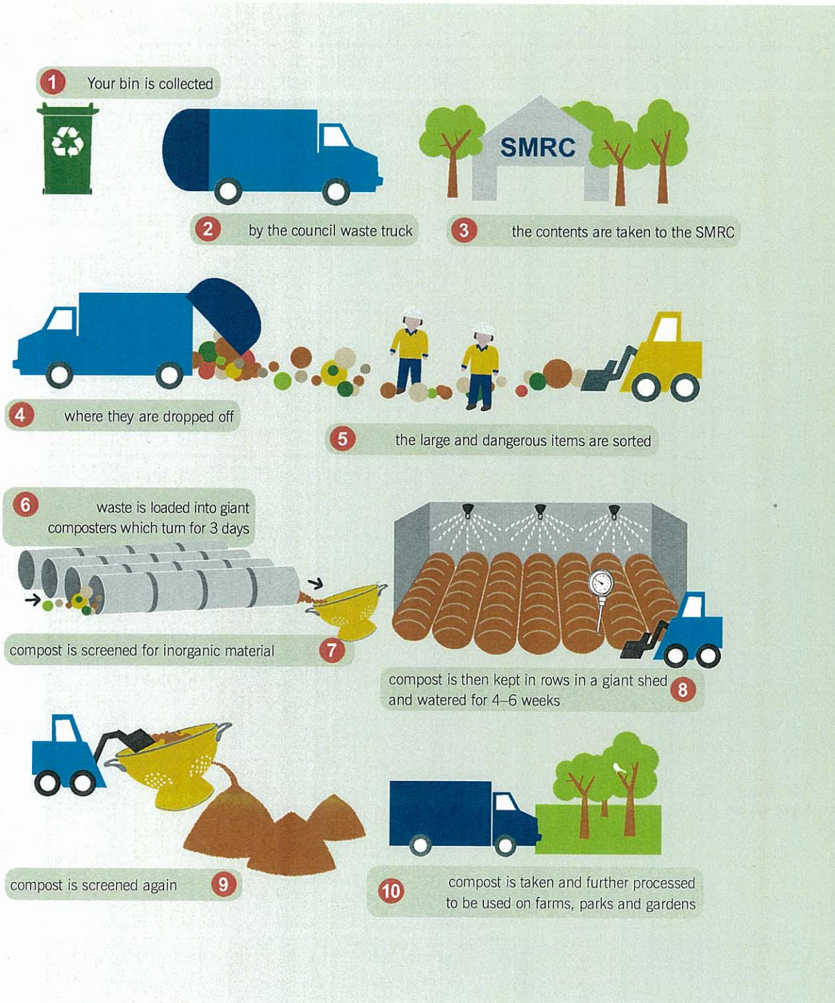
Figure 6: Green-top bin Resource Recovery Cycle at the SMRC (Courtesy SMRC, 2013)
