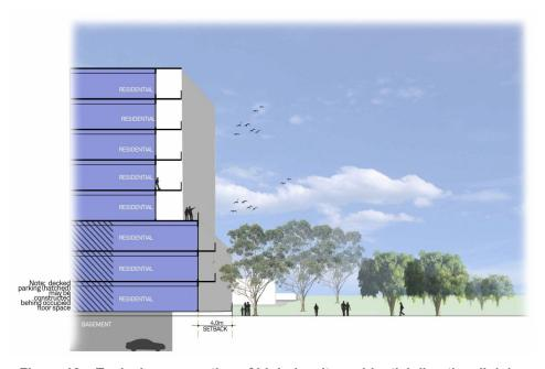
Figure 10 – Typical cross section of high density residential directly adjoining public open space
