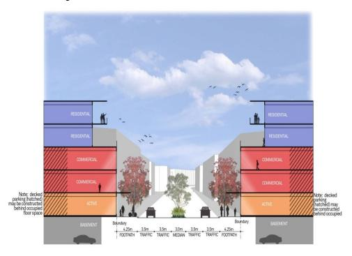
Figure 7 - Typical cross section for mixed use development
