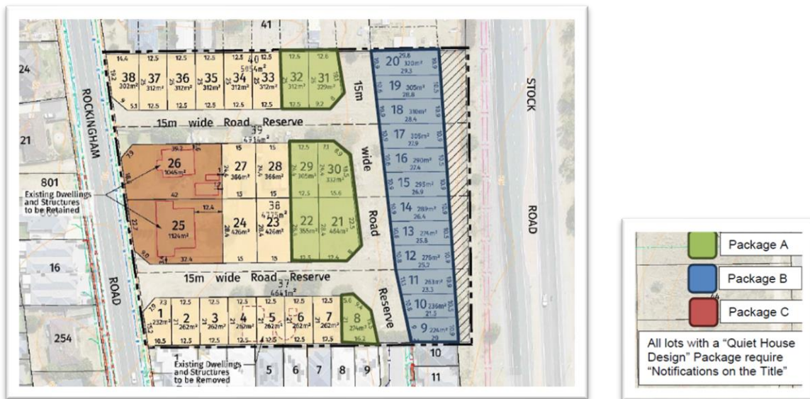
Figure 5 – Ground Floor Extent of required Quiet House Design packages (without a noise wall)
