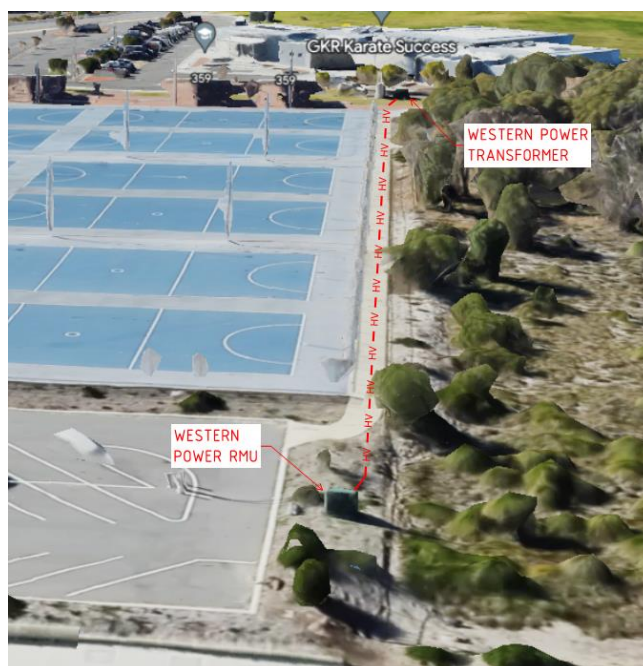
Image 3 - Indicative location of existing underground high voltage cable
