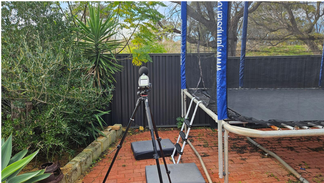
Figure 3-1: Photograph of Sound Level Meter on Site
