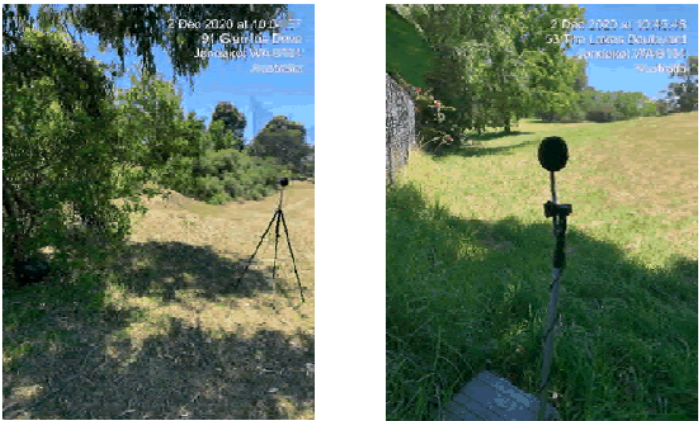
FIGURE 3.2 - NOISE MONITOR IN SITU
