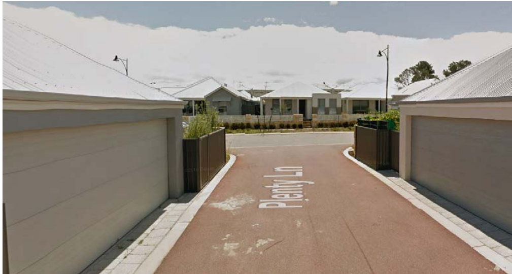
Figure 3 A dwelling has been centred to the laneway to allow direct line of sight from a habitable room down the length of the laneway
